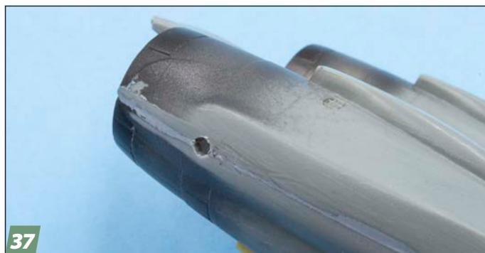
37 Once the halves were together, I drilled the holes for the horizontal stabilizers ...
