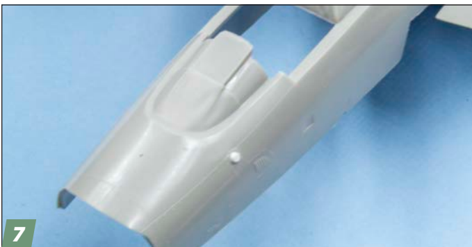
7 I filled a hole in the fuselage just under the windscreen designed to locate a probe — only early F-16As had this probe. I glued in similarly sized styrene rod and sanded it smooth.
