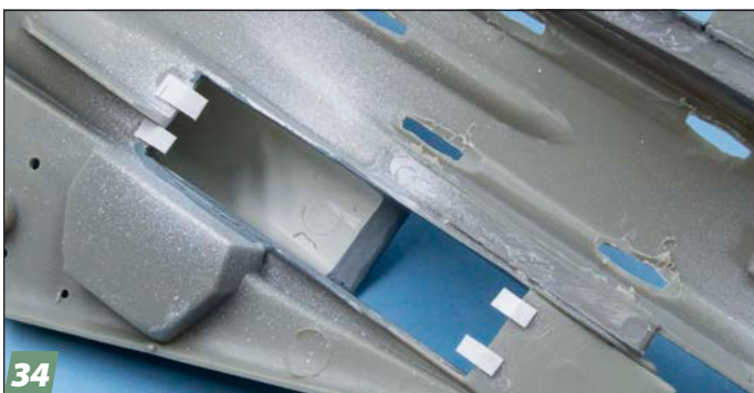
34 I painted smoothed seams and removed the tissue paper I had used to mask the fans. Now all I had to do was reattach the ramps; thin tabs made of thin styrene support the ramps and help keep them in place.
