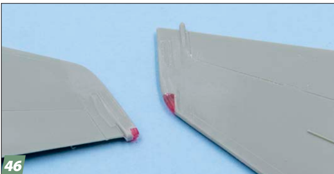
46 I repeated this method to improve the anti-collision lights on the vertical tails.
