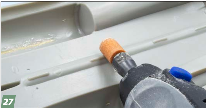
27 Flipping the lower fuselage over, I opened up the cavities for the AIM-7 Sparrow fins using a grinding stone in a rotary tool to remove the tops of the bays ...
