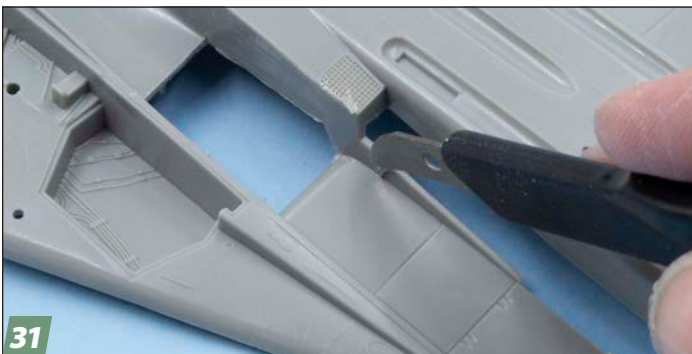
31 I usually close up the fuselage halves without worrying about the intakes because it is nearly impossible to eliminate the seams. This time, in a moment of insanity, I decided to see if I could overcome the fit problems. The main thing preventing cleanup of the intake seams was access, because the intake ramps are in the way. What if I removed the ramps? I began my little experiment by cutting away the ramps with a scribe.
