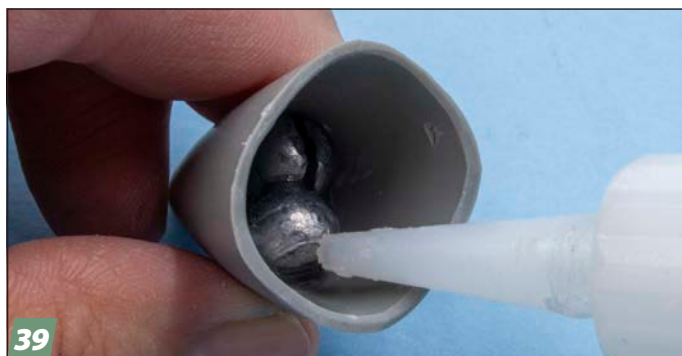
39 Although the model can stand on its gear without it, I always superglue a few small fishing weights into the nose to make sure the model doesn't become a tail sitter.
