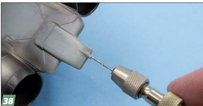
38 ... and hollowed out the fuel dump vent at the tail with a pin vise.
