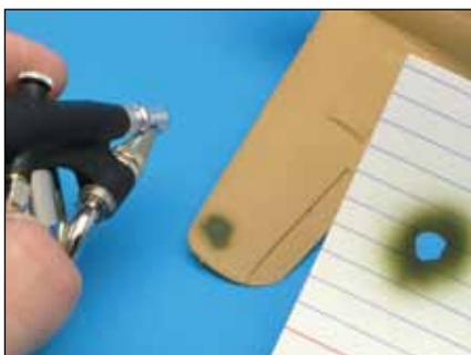
Despite the large burst of paint, only a small spot makes its way onto the model's wing through the hole in the card. By working slowly and applying the pattern a spot at a time, Matthew was able to apply the pattern precisely.
