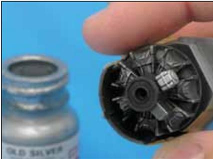
Not much of the 190's BMW 14-cylinder radial engine is visible inside the fuselage – a large cooling fan covers most of the opening. Matthew airbrushed the engine flat black, then dry-brushed it with Floquil old silver enamel (No. 110100) to highlight the cooling-fin detail.
