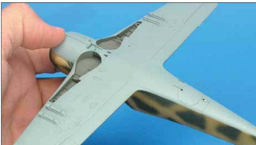
After a couple days of drying time, Matthew masked the model and applied the underside color, RLM 78 hellblau (Testor Model Master No. 2087). A hard line separates it and the upper-fuselage camouflage. When the hellblau was dry, he masked and painted the wheel wells gray.
