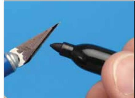
Trimming foil can be tricky. Matthew installed a brand-new No. 11 blade in his hobby knife, then blackened the blade with a permanent marker. The black finish cuts down on the reflections between the highly polished blade and foil and makes it easier to follow the line of the canopy framework during the trimming.
