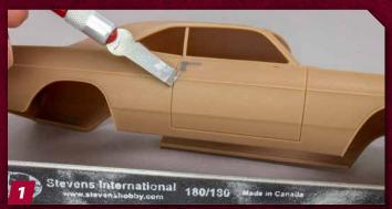
To remove the base-level trim from a 3D-printed 1969 Dodge Polara, I slowly removed about 75% of the trim with a knife. I kept the knife steady and worked my way along the body, careful not to gouge it. Then I sanded the area with progressively finer sanding sticks.
