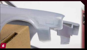
Using the in-cap applicator brush, I swiped the area and allowed 15 minutes for it to dry. The chemical reaction brought what's left of the emblem to the surface. Then I gave the area a final sanding and applied primer as needed. No ghost image this time! **FSM**
