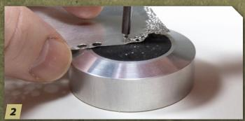
To make the rivets, simply press the punch through your chosen material (I'm using aluminum sheet) and leave them on the rubber block. The rivets are tiny and can be difficult to pick up with tweezers. But don't worry!
