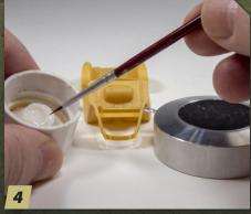
Position the rubber block close to the model and use the acrylic gel right from the cap after shaking the bottle. Wet the tip of the brush with a tiny amount of acrylic gel.
