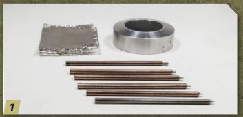
I use UMM-USA rivet punches and the hardened rubber block that comes with the UMM MultiShape Punch Set (No. UMM10). You can punch rivets out of thin aluminum sheet, plastic, or even photoetched metal.
