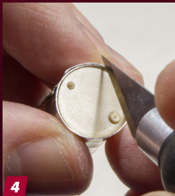
4 Wrap the foil around one of the drum ends and mark the overlap with a hobby knife. Then cut the foil to length using a metal ruler. If the details have gone a little soft, wrap the foil around your original pattern to sharpen them.
