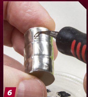
6 Flow superglue along the wall seam and carefully press it together. The foil bends easily, so light pressure will close the gap.
