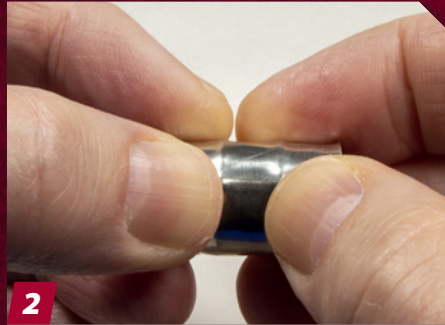
2 Wrap the foil strip around the drum and, with both hands, press the foil firmly onto the drum's sides to imprint the ridge pattern into the foil.
