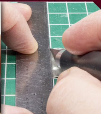
4 Wrap the foil around one of the drum ends and mark the overlap with a hobby knife. Then cut the foil to length using a metal ruler. If the details have gone a little soft, wrap the foil around your original pattern to sharpen them.
