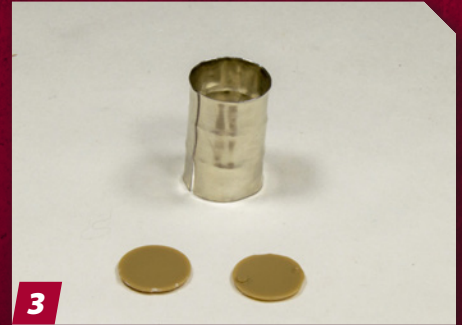
3 To make the drum's top and bottom, use discs cut or punched from styrene sheet that you can detail yourself or parts you may have in your spares box, as seen here.
