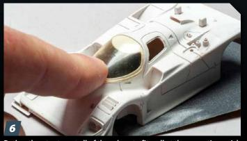
Rather than try to get all of the edges to fit well at the same time, pick one and shape it with 400-grit sandpaper. I worked the windshield's rear edges to fit the body, using one as a reference for the other. With those in place, there was a consistent fit for shaping the rest.
