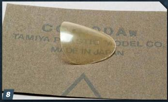
The windshield has been sanded to fit, but the plastic often has fuzzy remnants from the 400-grit sandpaper. Lightly sand the edges with 1000-grit sandpaper to eliminate the fuzz. You can also use the backside of a hobby knife to scrape the edges on thicker parts.
