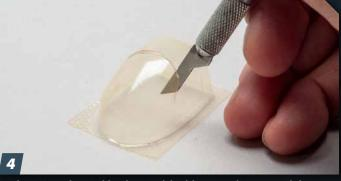
For big, curved parts like the windshield, score a line around the part, being careful not to cut into other parts. After several light passes, the knife will cut through. Do not bend or twist the plastic more than needed because it can crack, tear, or kink — no scissors yet!
