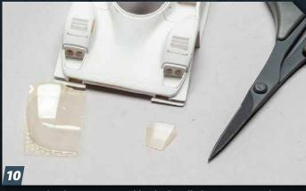
For parts that have no curves, like the headlight covers, trim them with scissors and fine-tune them with sandpaper as before. I find fitting the front and back edges first works well to provide conistent alignment to trim the angles on the sides. You don't want any gaps.
