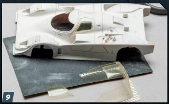
Small curved parts have less chance of crimping, so you can cut them out with scissors. Place each over its opening and trim the top, rear, and bottom edges. Sand the rear and bottom edges to fit, and then the top. Use the Sharpie method above to fit the front edge.
