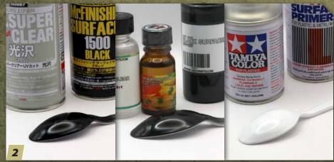
I coated each primer with its corresponding clear: Mr. Super Clear UV Cut (No. B522) from the spray can, Splash 2K Ultra Gloss Clear (No. SP-UC1) through an airbrush, and Tamiya Gloss Clear (No. TS-13) from the can.
