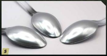
After a third mist coat, the spoons appear chrome, and they all have the same color density regardless of the base-coat color. According to SMS, you can apply more coats to get the coverage and effect you're looking for. But we aren't finished yet.
