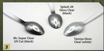
Shake the SMS Hyperchrome well. There isn't an agitator inside, so don't expect to hear one rattling around. I pour the Hyperchrome directly into my airbrush cup, set my air pressure to 25 psi, and mist the paint on. Here's the result after one coat on each spoon.
