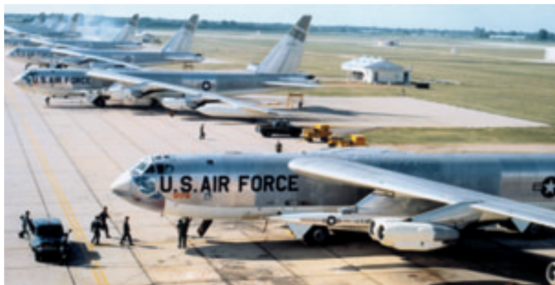
6 Still going strong more than 50 years after its first flight, Boeing's B-52 Stratofortress is possibly the most famous jet bomber in history. These F models carried Hound Dog cruise missiles. USAF photo via Wayne Mutza
