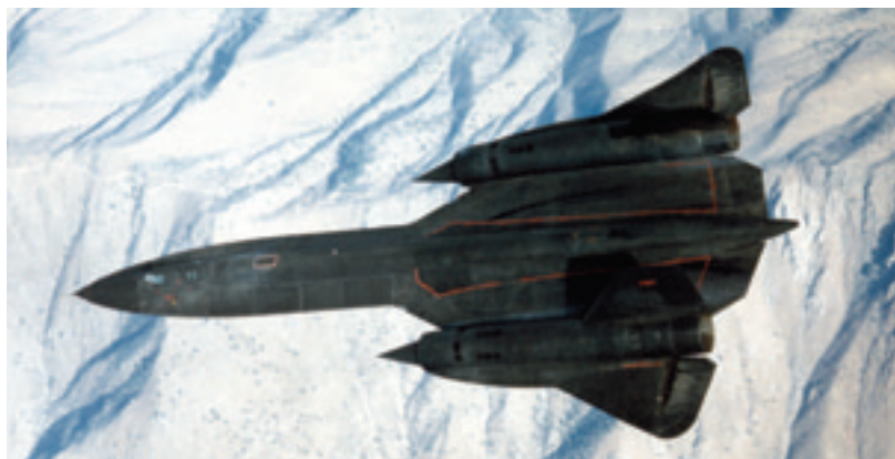
7 The famous "Blackbird" – Lockheed's SR-71A. Nearly 40 years after its first flight, it is still unmatched in performance. Mach 3 at 80,000 made it untouchable. USAF photo via Jim Goodall
