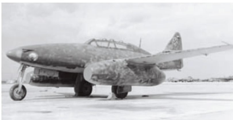
3 Messerschmitt's revolutionary Me 262 was the first jet fighter to see action. This captured two-seater was photographed at Wright Field, Dayton, Ohio, in March 1946. Jim Hawkins photo via Len Lundh
